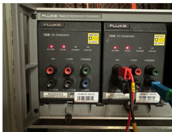
Figure 8: Voltage standard Fluke 732B used for 1V calibration
