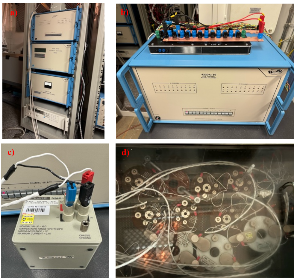
Figure 6: Measurement setup. a) automatic resistance bridge and low thermal EMF scanner, b) second scanner and measured transfer standard, c) portable standard resistor Fluke 742A-10 d) CERN reference resistors in oil bath
