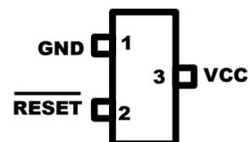
These and similar ICs come almost invariably in the tiniest SMD packages, typically in SOT-23. One of the few through-hole-packaged "three-leg" reset circuit is the MCP100/101 combo manufactured by Microchip.
