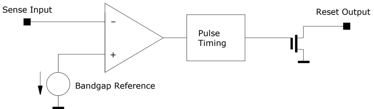
The reset output gets active immediately after the comparator senses drop in the input voltage and remains active until the supply/input voltage regains the proper value plus a predetermined time period. Some reset circuits (usually the integrated) feature short glitches suppression, so they won't trip if the voltage drops below the trigger level for a very short time (to provide extra noise immunity).
