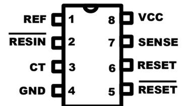
There is also a CMOS variant of the 7705, often carrying the letter C either in the middle of numbers or in the prefix. It has a lower power consumption, works from lower supply voltage (around ), but note that its active-high output is push-pull.
